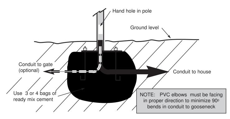
DETAIL OF ATTACHMENT OF POLE ONTO BASE
