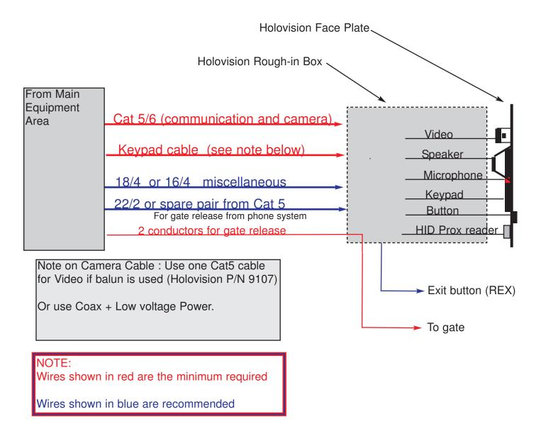
Wire for gate release from phone system is required, but it can be a spare pair from Cat5/6
