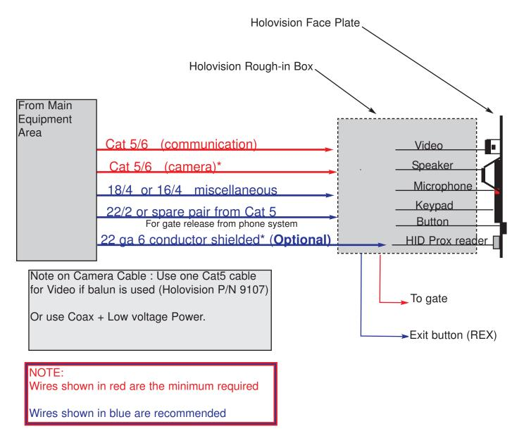
Wire for gate release from phone system is required, but it can be a spare pair from Cat5/6
