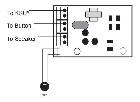
To use the Door Intercom Unit, connect to the KSU as shown above.
