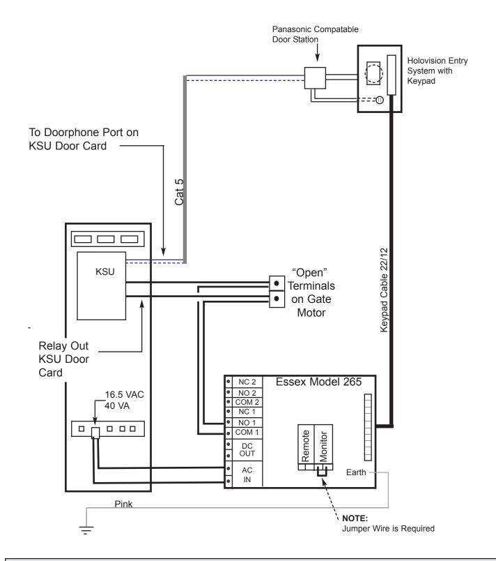
NOTE : Remove the jumper wire & MOVs from left side terminal strip. Wire right side terminal strip "color for color".
