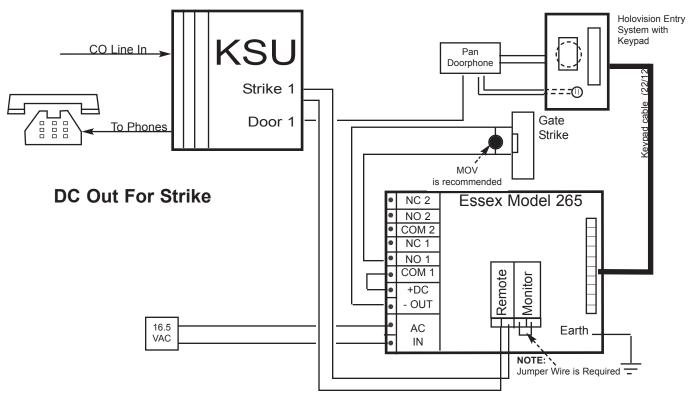
The 265 module comes with jumpers and MOVs prewired to the left side of the terminal stirp. Remove all wires from left side of terminal strip and wire per this diagram
