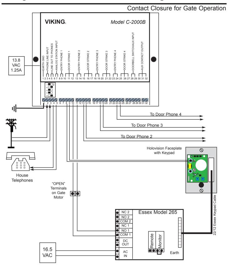
NOTE 1: Remove the jumper wire & MOVs from left side terminal strip. Wire right side terminal strip "color for color".
