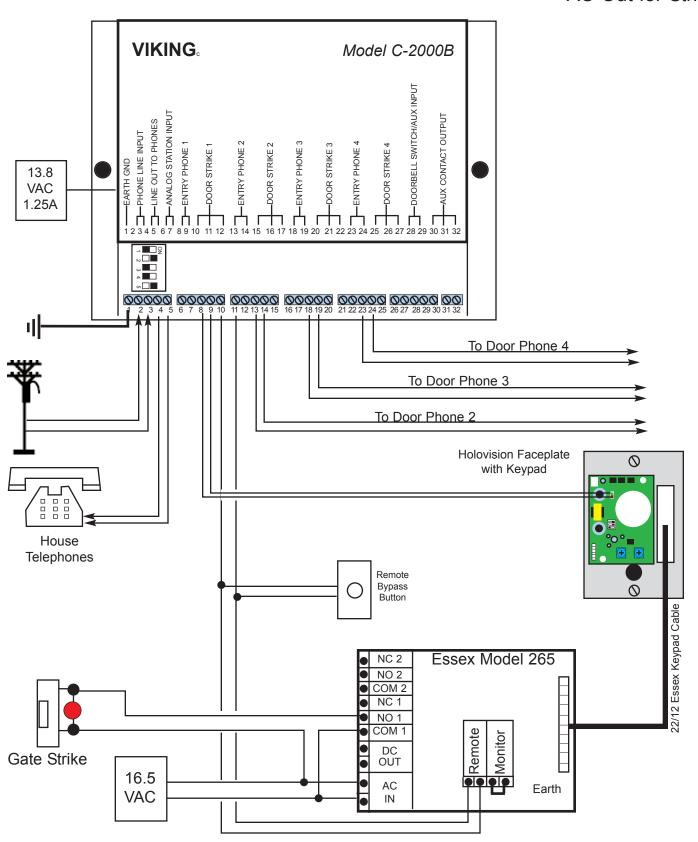
NOTE 1: Remove the jumper wire & MOVs from left side terminal strip. Wire right side terminal strip "color for color". NOTE 2: MOV (metal oxide varistor) is the small red component which is included. Its purpose is to absorb "inductive kick back" which can be created when power is removed from the strike.
