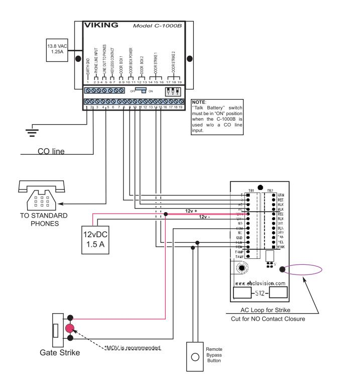
NOTE: MOV (metal oxide varistor) is the small red component which is included. Its purpose is to absorb "inductive kick back" which can be created when power is removed from the strike. Loop is required from 12v positive to contact common for DC power to strike.
